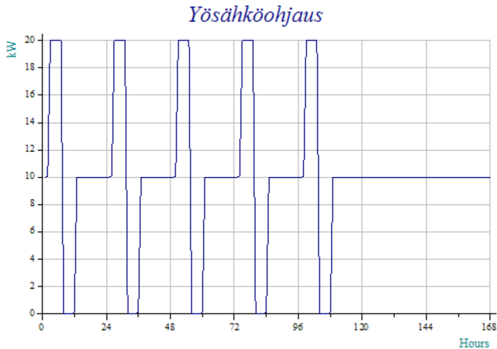
Fig 16. Optimised load when ToU tariffs are in place for both energy and distribution favouring night-time loads.
