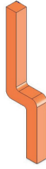
Figure 1: Equal channel angular pressing die used for producing the ultrafine grained structure.
