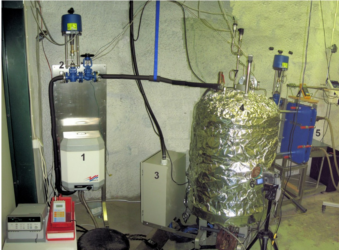
Fig. 2. COOLOCE experimental set-up: 1) feed water pre-heater, 2) feed water control valve, 3) connection box for the heaters, 4) pressure vessel, 5) steam line condenser and scale, 6) sightglass with video monitoring, 7) water level and pressure gauges.
