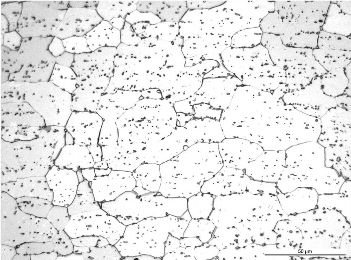
Fig. 22. The microstructure of alloy 450 after 5000 h of exposure.
