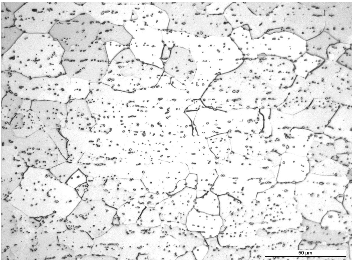
Fig. 21. The microstructure of alloy 430 after 500 h of exposure.
