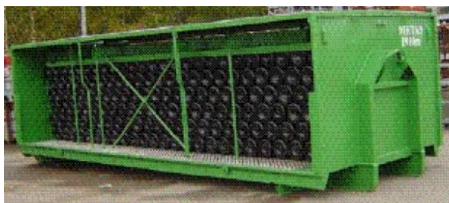
Figure 19. Hook-lift trailer (Sweco 2005).
