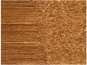
1.4162, Single straight laser weld
