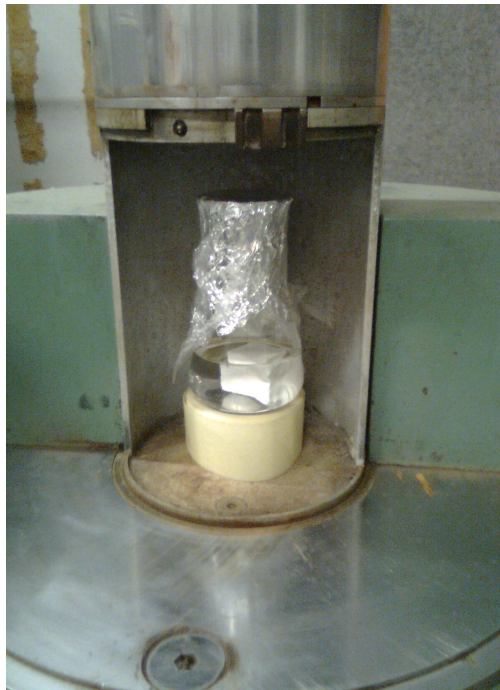
Figure 1. The position of concrete block sample in Gammacell 220 ready for irradiation.
