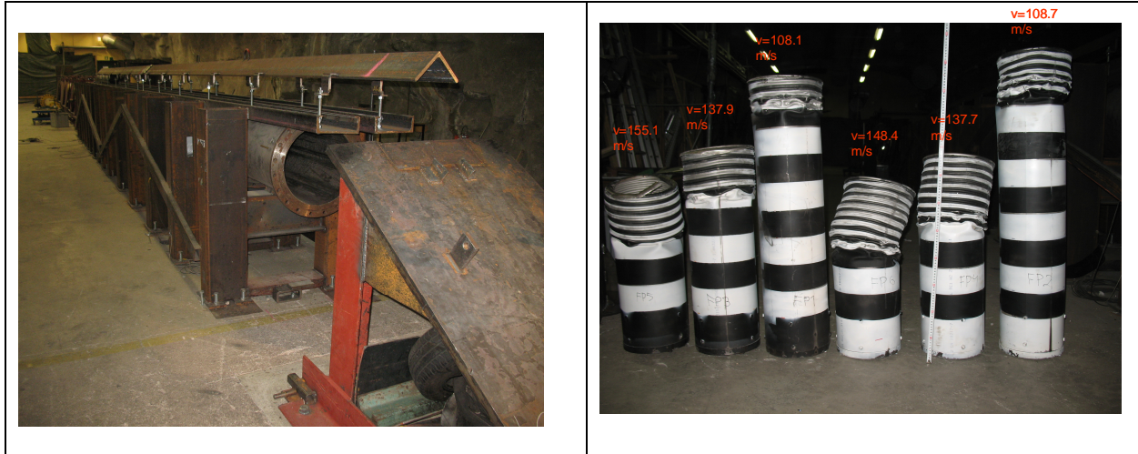
Fig. 1. Corner profile installed on top of acceleration tube (left). Stainless steel missiles after shooting (right).
