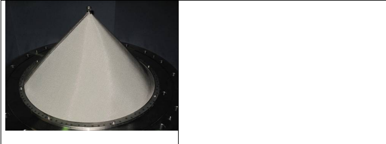
Figure 13. Heating arrangement of the COOLOCE test facility (top left), the test particle bed ( \varnothing 50 cm) held in the conical shape by a wire net (bottom left) and a void fraction prediction within the conical particle bed by PORFLO (right).
