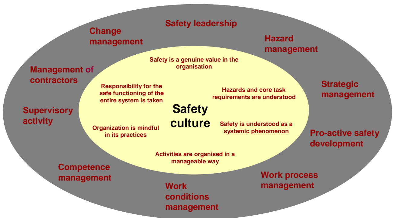
Figure 1. The DISC-model depicts the six safety culture criteria (in the middle) and the organisational functions which are necessary to in any safety critical organisation to fulfil the criteria.
