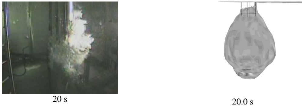
Figure 1. A gas bubble in water pool in an experiment performed in the CONDEX project. On the right, iso-surfaces of void fraction in CFD simulation are shown.
