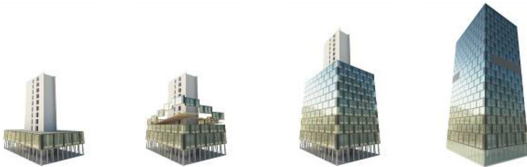
Fig. 1 LifeCycle Tower – construction phase
