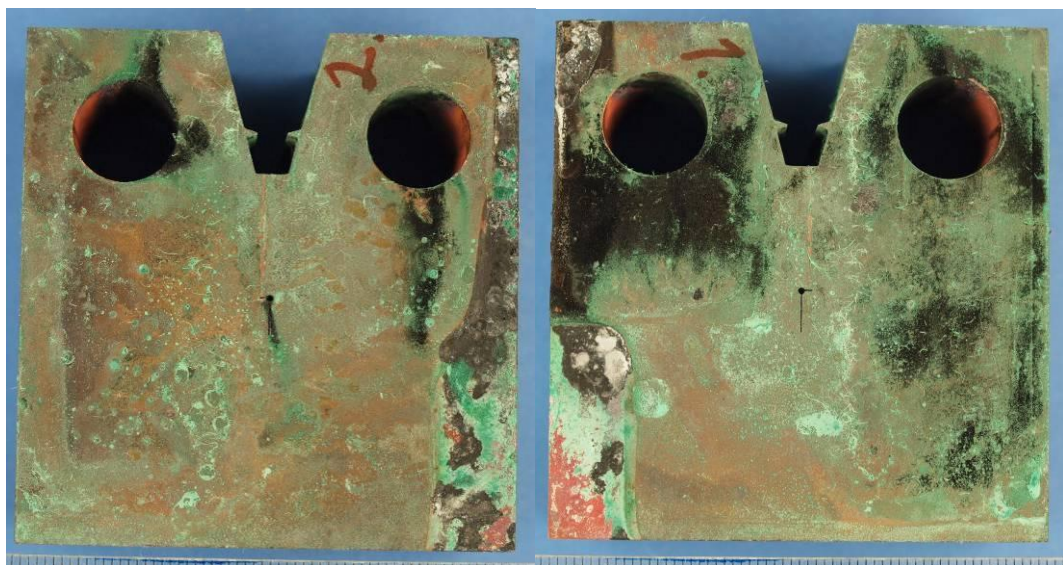
Fig. 14. The outer surface of the specimen FSW L75-2 after the corrosion experiment in saline water at a plane stress reference stress of 55 MPa at 90°C
