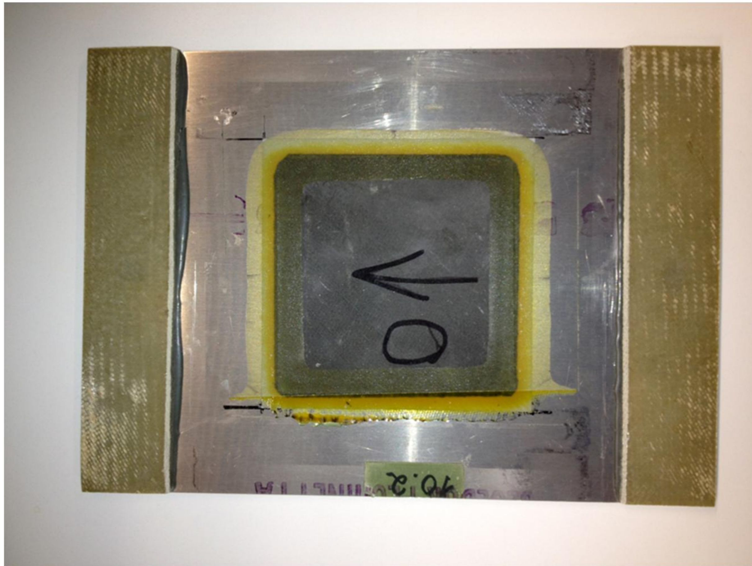
Figure 30: The examined structure; a 2024-T3 aluminum plate and a carbon/epoxy prepreg patch bonded with FM73M epoxy adhesive. Picture by courtesy of Aalto University.
