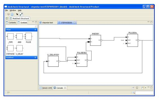
Figure 2. The Simantics modelling tool allows the user to specify the function block diagram in a graphical view, and generates the corresponding input file for the NuSMV model checker.
