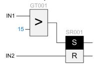
Figure 1. An exemplar fragment of a function block diagram with two connected blocks.
