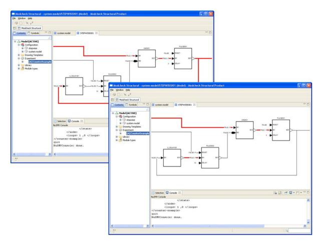
Figure 3. The counter-example output by the model checker is presented to the user as an animation illustrating how signal values change – a "living" function block diagram.
