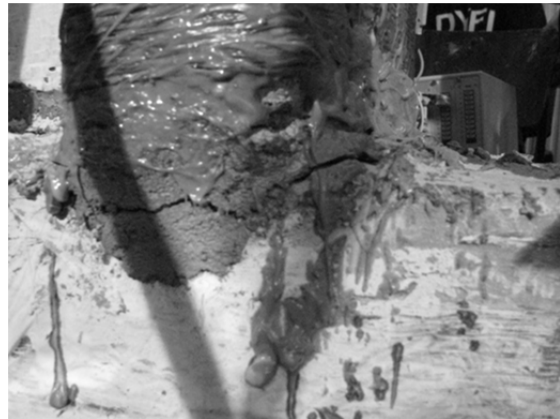
Figure 24. Cast in place mortar crush
