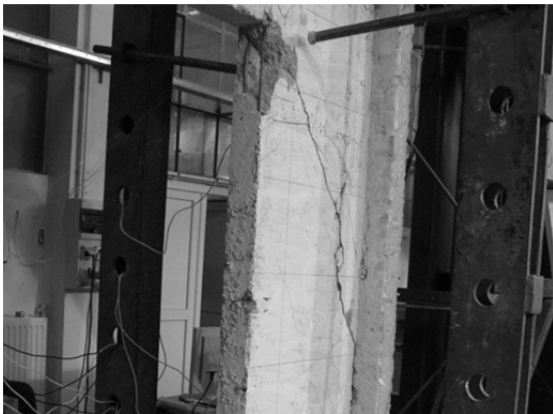
Figure 19. First diagonal crack in the right pier
