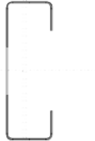
Figure 3: Effective section of Lipped channel 24.0x72.0x15.0 1.0 mm
