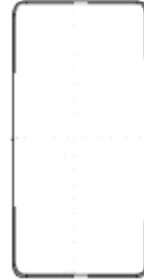
Figure 1: Effective section of Lipped channel 36.0x72.0x15.0 1.0 mm
