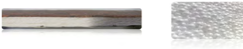
Figure 10. On the left, biofoam made out of cellulose fibres. On the right, ultra-light weight cellulose-based material.
