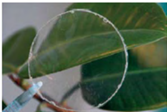
Figure 22. A transparent and flexible film obtained from a butylated and allylated xylan.
