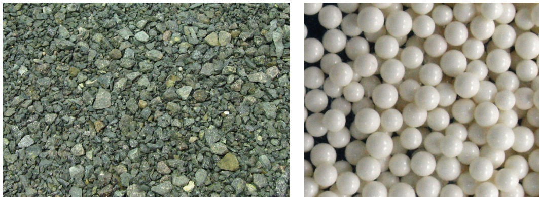
Fig. 1. The alumina gravel used in COOLOCE-8 (left) and the zirconia/silica beads used in COOLOCE-3 – COOLOCE-7 (right). Note: the scale of the images is not the same.
