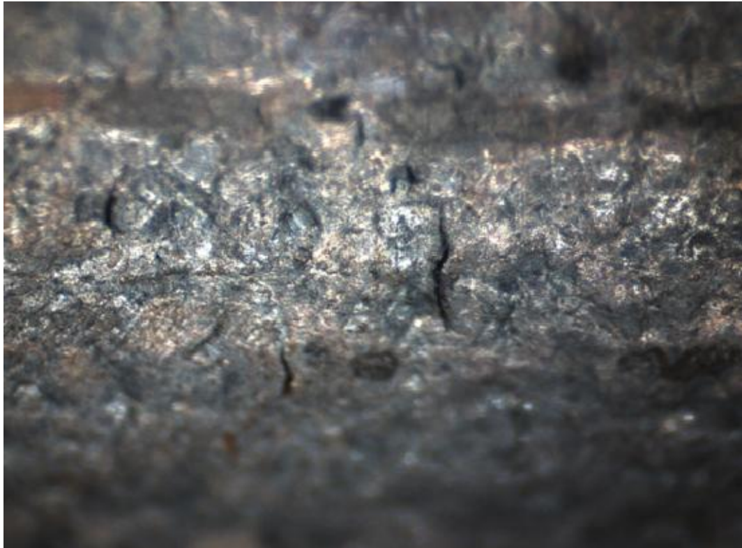
Fig. 3. Surface cracks in the uniaxial specimen V1 after 91 148 h at 120 MPa 150°C
