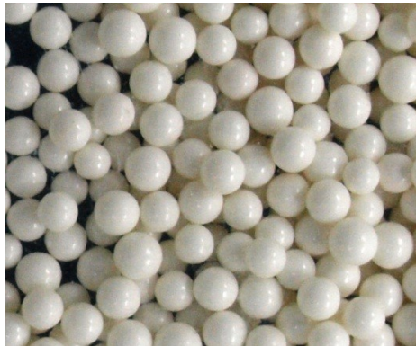
Fig. 3. Ceramic beads used as debris simulant.
