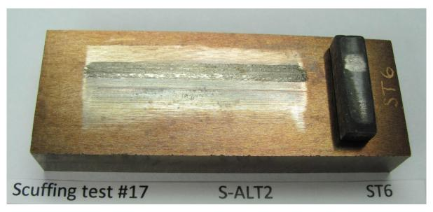
Figure 31. Example of a sample combination after a scuffing test (Test #17).
