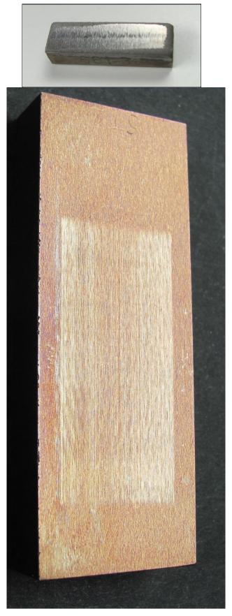
Figure 27. Example of a piston ring sample and cylinder liner plate sample combination after a running-in test (Test #2).
