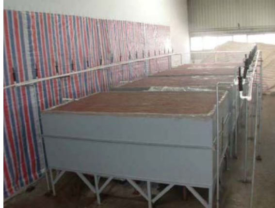
Figure 16. A Porous pavement test cells. [Hou et al. 2008]
