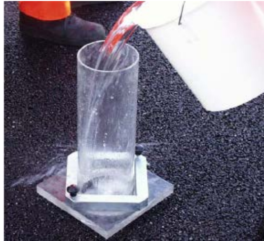
Figure 8. Becker's tube which is used for measuring the permeability of porous pavements. [Haider et al. 2008]
