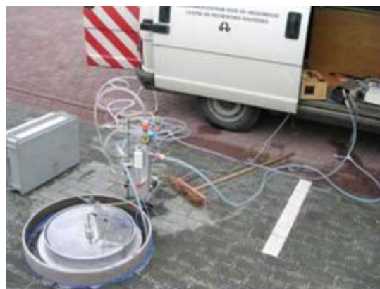
Figure 6. A Double-ring infiltrometer for the measurement of PICP. [Beeldens et al. 2009]
