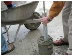
Second lift compacted
