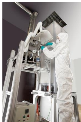
Figure 2 – VTT Pilot unit TIPU for synthesis of metallic nanoparticles
