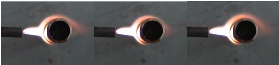
Figure 10. Snapshots of flame heating a copper pipe (above) showing fluctuations of the flame. Single hole burner, distance between burner and pipe of diameter 5/8" is 15 mm, H 2 flow rate 6 liters per minute.
