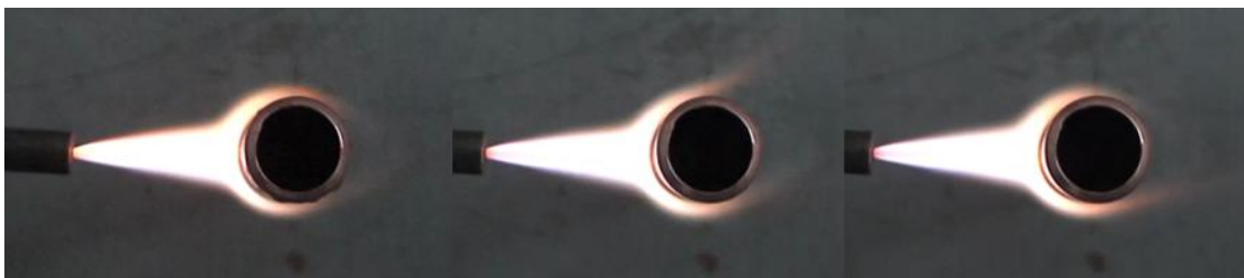
Figure 11. Snapshots of flame heating a copper pipe (above) showing fluctuations of the flame. Single hole burner, distance between burner and pipe of diameter 5/8" is 30 mm, H 2 flow rate 6 liters per minute.
