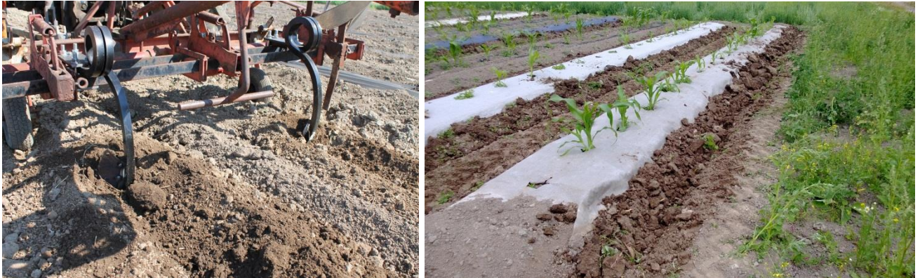
Figure 27 A modified sugar beet hoe for hilling up the edges of mulch (left). A row of maize which has been hilled up with the modified hoe (right).
