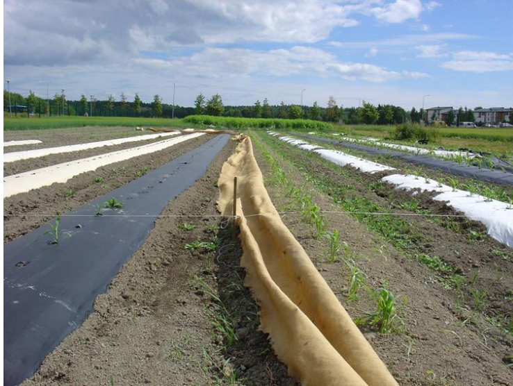
Figure 8. An experimental paper mulch of which the soil buried edges are degraded thereby allowing wind to tear the paper from the ground (Agripap-field, Viikki, 2011)
