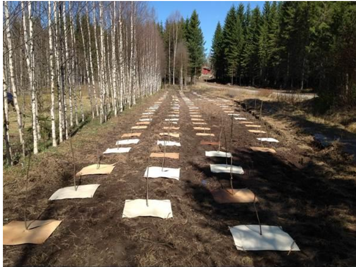
Figure 15. Paper board mulch sheets in forestation use. Agripap-field test site in Pieksamäki.
