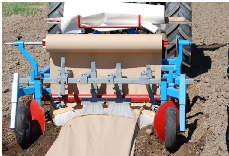
Figure 34 Press wheels replaced with nylon brushes
