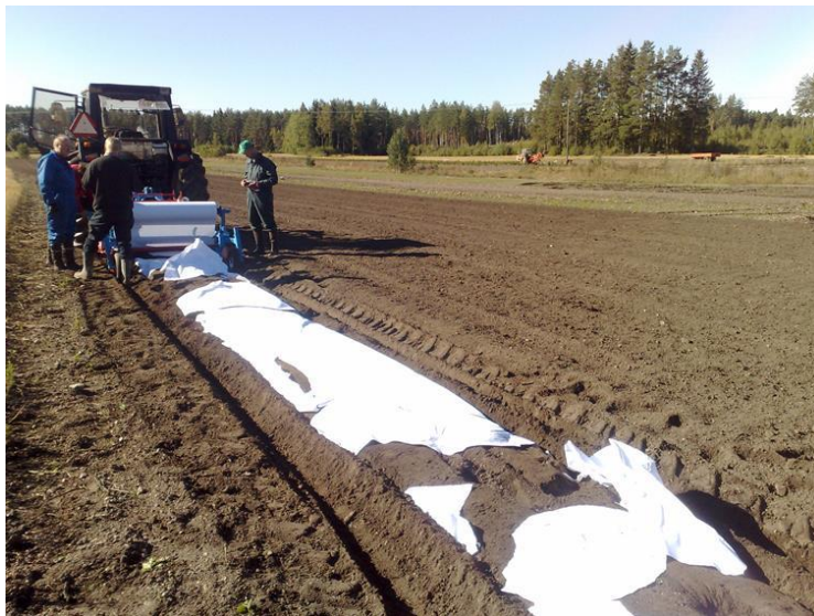
Figure 9. Breakage of non-extensible paper in mechanized laying. (Laitila, Avagro, Agripap-field, 2010).
