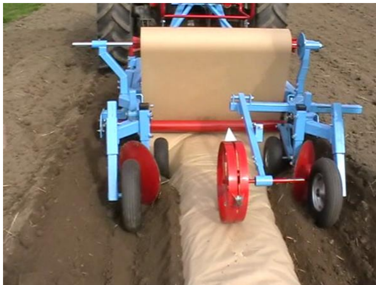
Figure 24. A standard Rapi laying machine (Avagro Oy) laying successfully mulch made of sack paper
