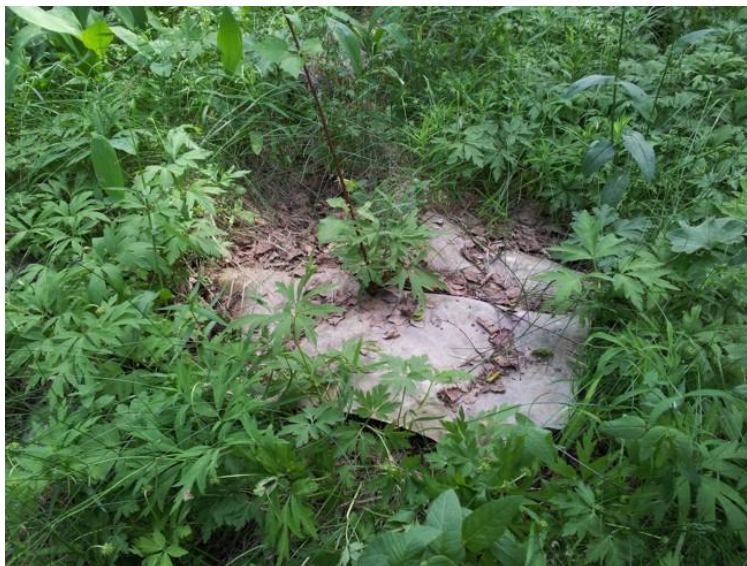
Figure 33. Heat treated PGW board after one year.
