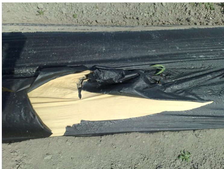
Figure 30. Biodegradable plastic film coating peeling off after two weeks.
