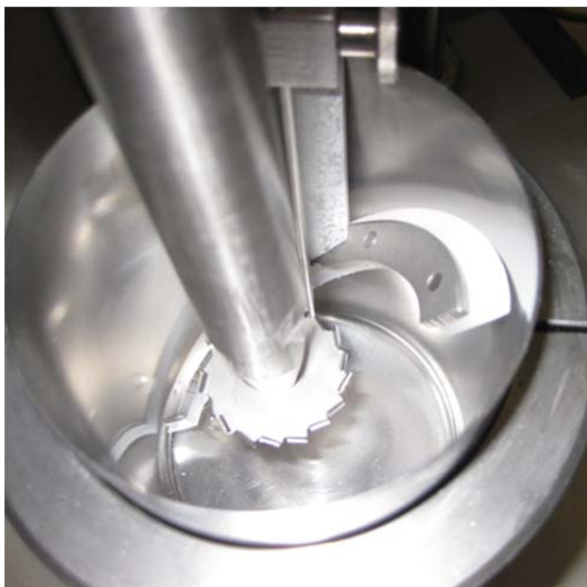
Figure 5. Dispermat mixing system with scraper tool. Pastes with high viscosity can be mixed and dispersed.
