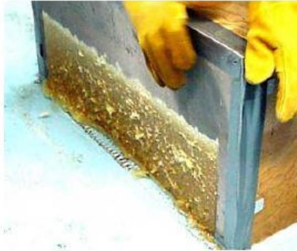
Figure 1. Typical accumulation of fine debris bed on the strainer (NEA, 2013).
