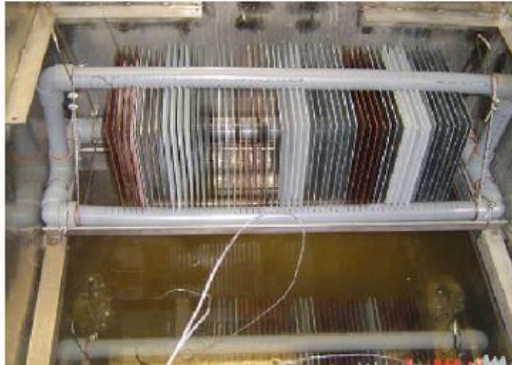
Figure 10. Metal, concrete etc. loaded on racks in ICET test tank. (Dallman et al., 2006a)
