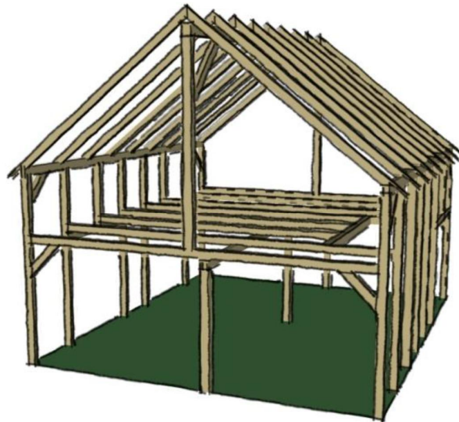
Figure 15. Example of a timber building frame ( www.timberhart.com ).
