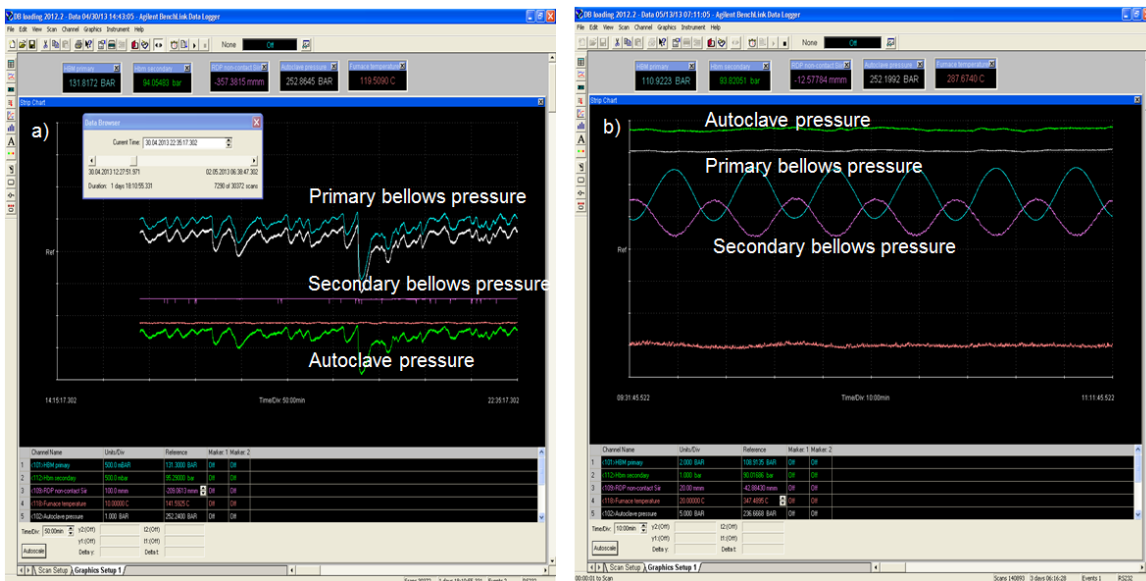
Figure 19. The pressure synchronization during the test, a) constant load and b) cyclic load.
