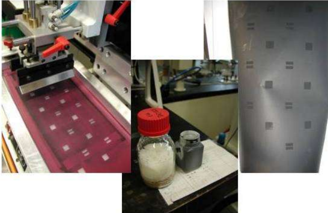
Figure 4.13. Semi-automatic screen printer and IL containing ink + print with AC and Reline.
