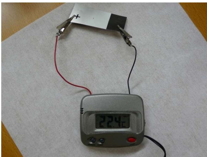
Figure 3.3. Supercapacitor having a gel electrolyte could be charged to 1.5 V and used as a power source for a digital thermometer.
