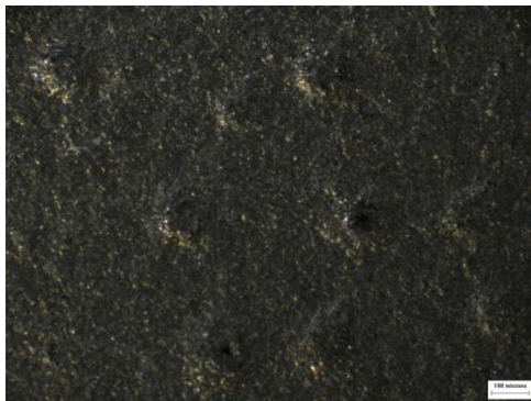
Figure 4.15. Light microscope photo about microblistering on the surface of printed Walki C2S. Too intensive drying created the microblistering. Evaporable moisture broke the surface of thick graphite ink layer and produced even pinholes. This observation forced to decrease the drying temperatures.
