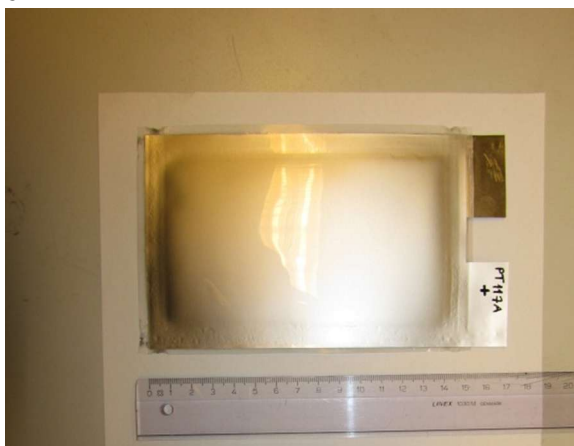
Figure 5.2. Supercapacitors (about 50 x 70 mm) made on Al/PET-substrate (a), Walki Al/paper C2S (b), Stora Enso Lunchbox Al/cardboard (c) and titanium coated aluminium foil (d). Supercapacitor (about 100 x 150 mm) made on Al/PET-substrate (e) and titanium coated aluminium foil (f).
