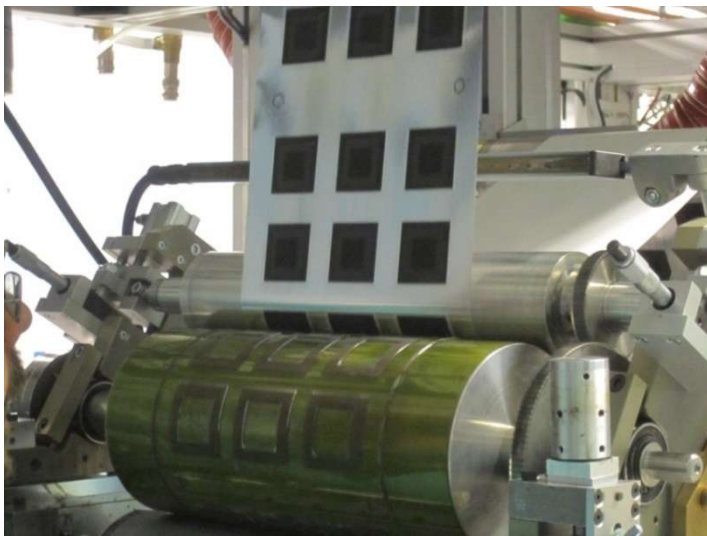
Figure 4.12. Flexo printing unit during the application of Aquaseal layer. Flexo printing worked well with Aquaseal liquid since it was originally developed for flexography.
