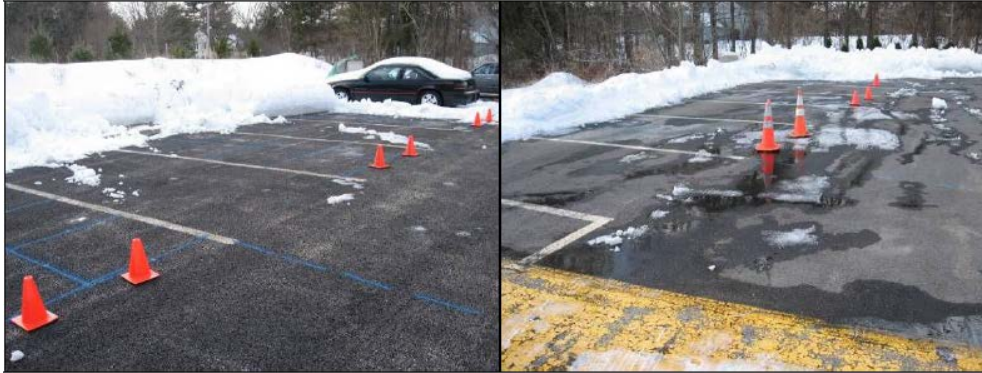
Figure 12. Instantaneous pavement conditions after thawing and refreezing of meltwater. a) Porous asphalt; b) Dense asphalt. [Houle 2008]
