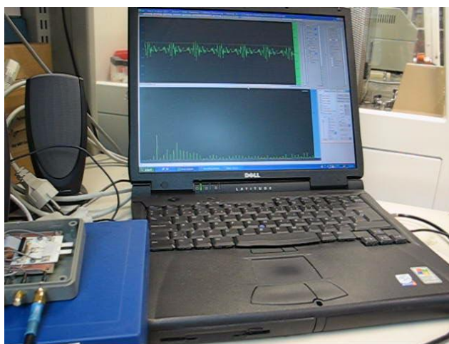
Fig. 3. Frequency modulated continuous wave (FMCW) radar demonstration with Infineon's RX/TX chip on LCP platform.
