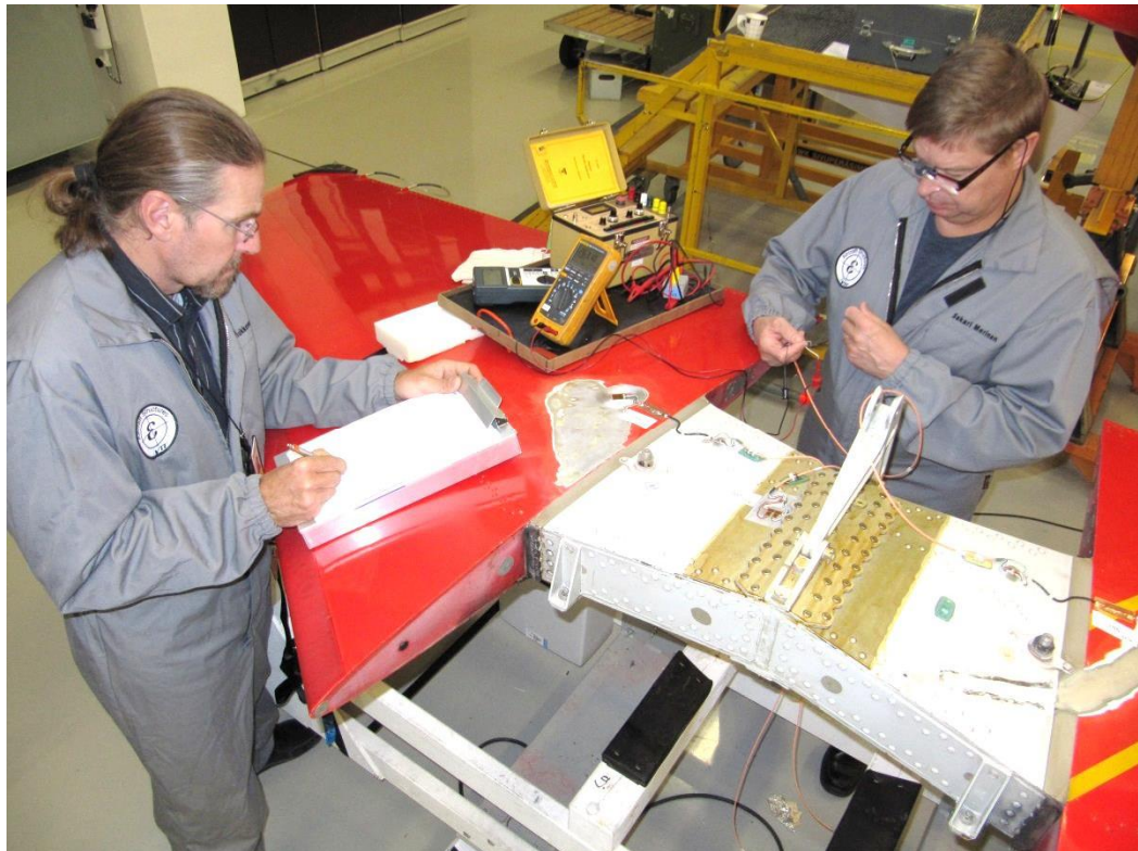
Figure 12: An overview of Mk66 tailplane mini OLM instrumentation. Picture by courtesy of VTT Ltd.
