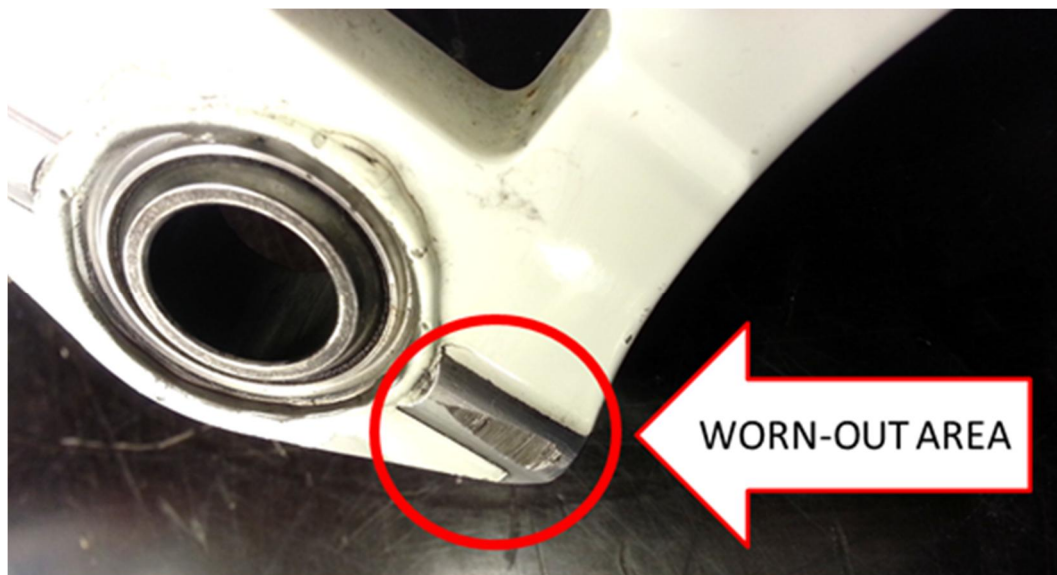
Figure 20: An overview of the Aileron's hydraulic cylinder's worn flange. Picture by courtesy of the FINAF.
