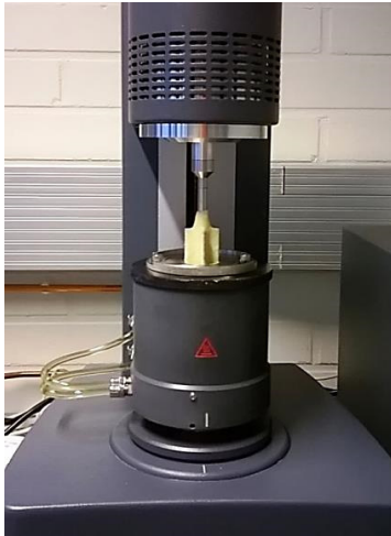
Figure 12. Viscosity determination of fermented faba bean sample with reometer.
