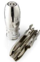
Fuel injector for jet engine Complex design printed as one piece, cost - 40%, weight -50% (EOS & Morris technologies)
