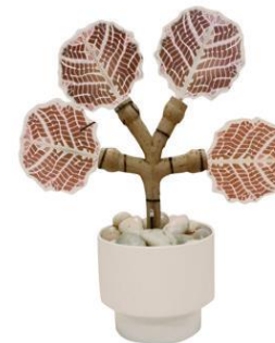
Energy harvesting tree Prototype of 3D printed artificial tree for energy harvesting (FDM)
