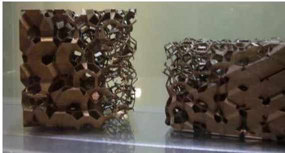
Internal structures of solid object To achieve desired strength properties with less weight
