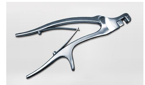
Surgical guide Prototype of a Plate Bender, used to contour plates for spinal surgery (DePuy Spine)
