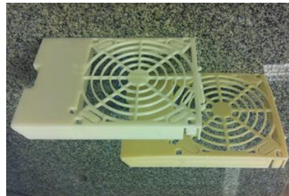
Housing for fan 3D printed housing for fan, difficult to manufacture conventionally (FDM)
