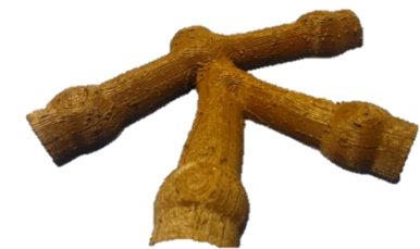
Biocomposite branch Artificial branch 3D printed from experimental biocomposite (FDM)
