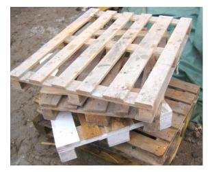
Figure 5. Example of class B wood, a pallet. Photo  $\ensuremath{\mathrm{VTT}}$
