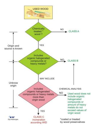
Figure 3. Flow chart how to determinate different used wood categories
