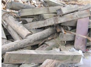
Figure 7. Example of class D wood. Photo, VTT.
