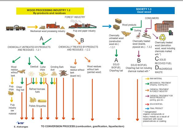
Figure 2. Classification of the industrial by-products and residues and used wood to A, B, C and D classes [2].
