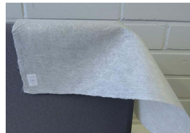
70% 12 mm viscose fibres, 30% softwood kraft pulp 50 g/m 2 Tensile strength 207 N/m Strain at max force 26%
