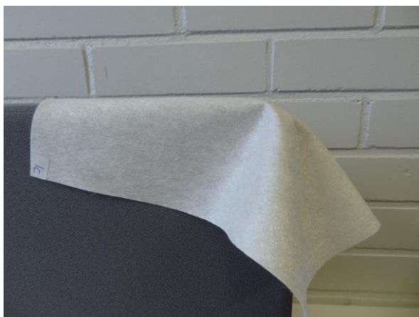
100% 24 mm viscose fibres 150 g/m 2 Tensile strength 128 N/m Strain at max force 10%
