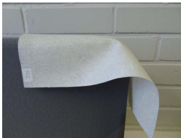
100% 12 mm viscose fibres 100 g/m 2 Tensile strength* 834 N/m Strain at max force 36%
