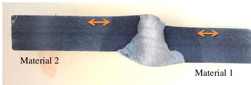
Figure 6. Macrograph of a cross-section close to the cracked region after oxalic acid etching. A clear mis-alignment between the pipes is seen. The region where grain boundary attack was observed in the two materials is indicated in the picture.
