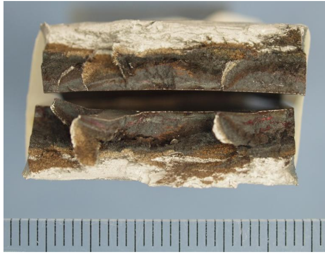
Figure 3. Photograph of the fracture surface of a part of the crack in material 1.
