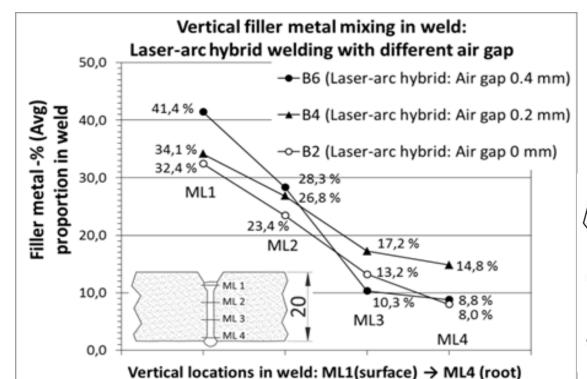
Laser-arc hybrid weld
