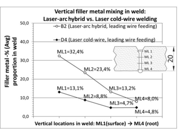
Laser-arc hybrid weld vs. laser cold-wire Basemetal AISI 316 (17.6 % Cr Filler wire 2205 (22.9 % Cr)
