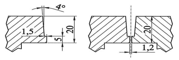
Multi-pass weld by 3 kW Nd:YAG 20 mm, laser-arc hybrid
