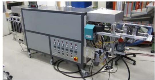
Figure 1. Tubular furnace for carbonization of electrospun sheets.
