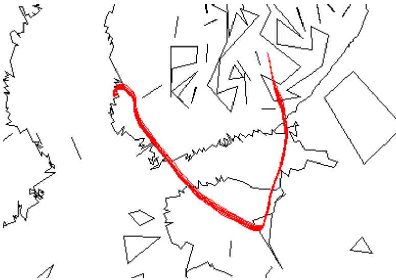
Figure 8.2. Advection in case 23567, described by 8 trajectories starting during 3 hours, calculated by VALMA using single-point wind measurements. Note: Weather data is reliable only near the source. Initial spread direction is north (low wind speed), after which the plume turns clockwise through east towards south-east, in the direction of Turku.
