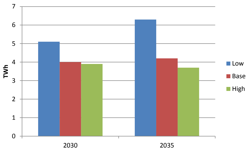
Figure 18. Condensing power production in the Nordic market area in selected scenarios according to model calculations.
