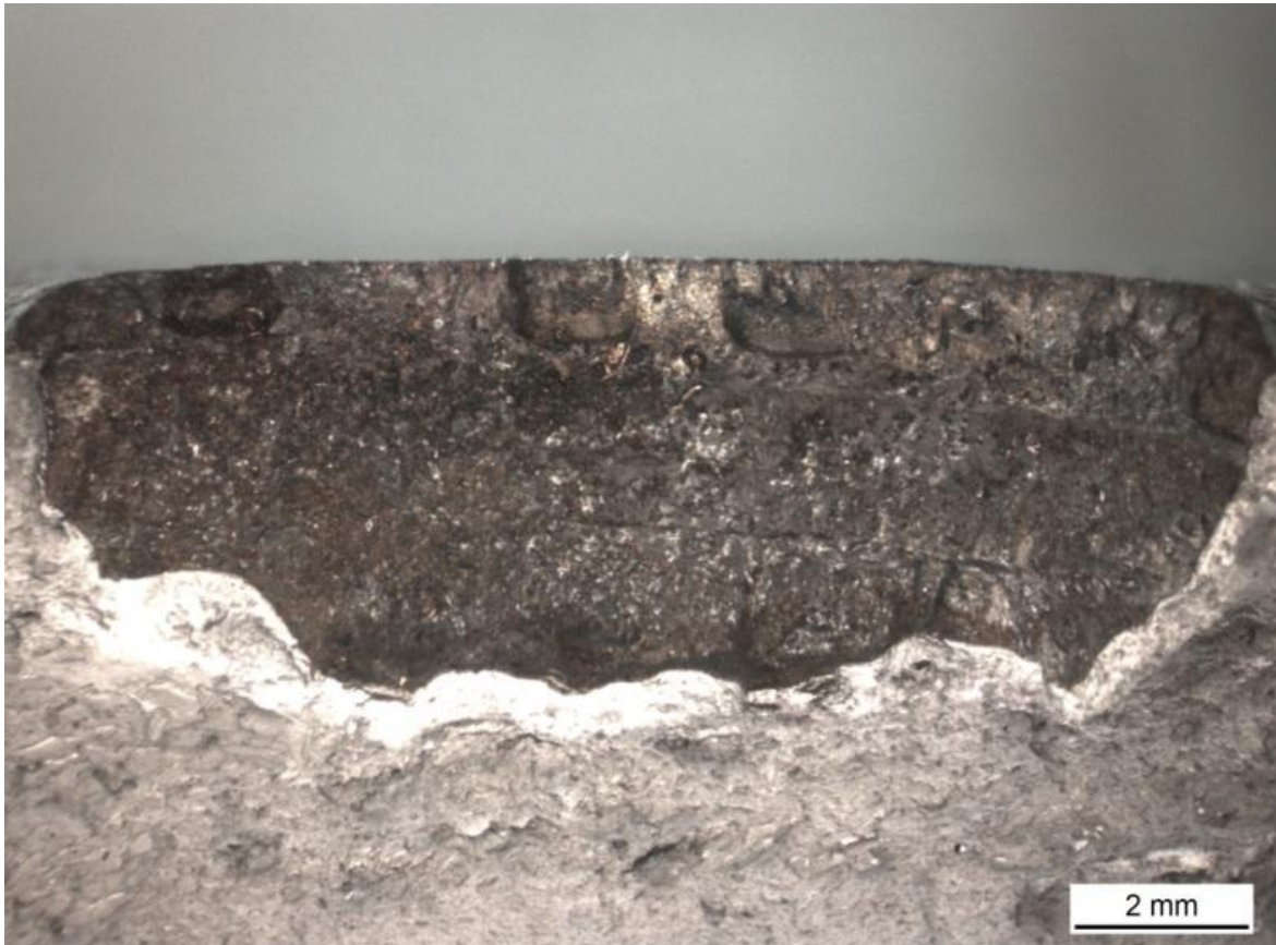
Figure 10. Photograph of the surface of the crack in test piece MF B. [1]
