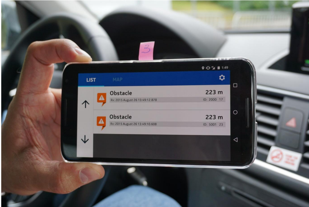
Figure 7. Acknowledge from short (HERE) and long loop (Infotripla) to a mobile phone initiated warning, therefore user sees two messages.
