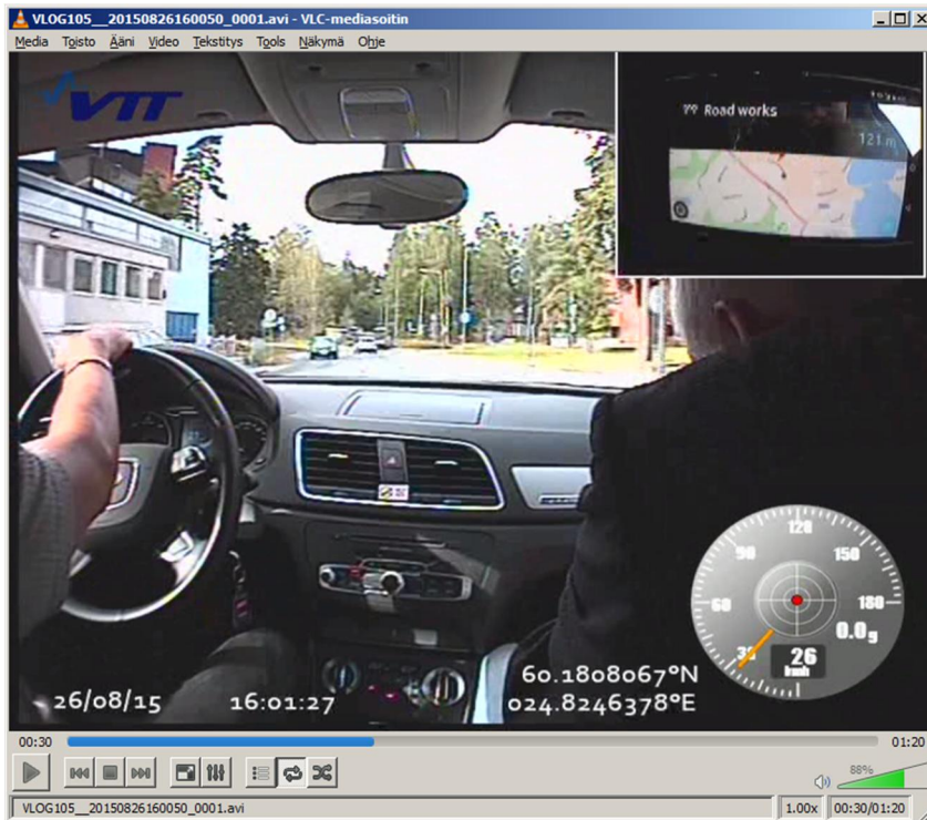
Figure 10. VBOX video with inlayed timestamp, coordinates, speed, acceleration and M5 user interface
