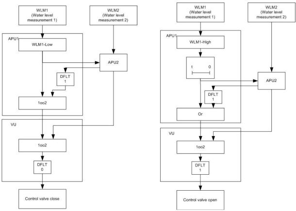
Figure 3. The control logic of the example system
