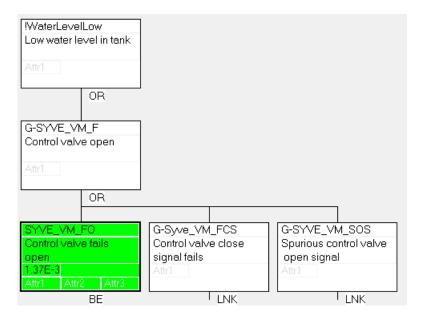
Figure 5. Master fault tree for top event low water level in tank.
