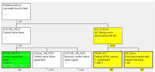
Figure 6. Master fault tree for top event low water level in tank including design error.
