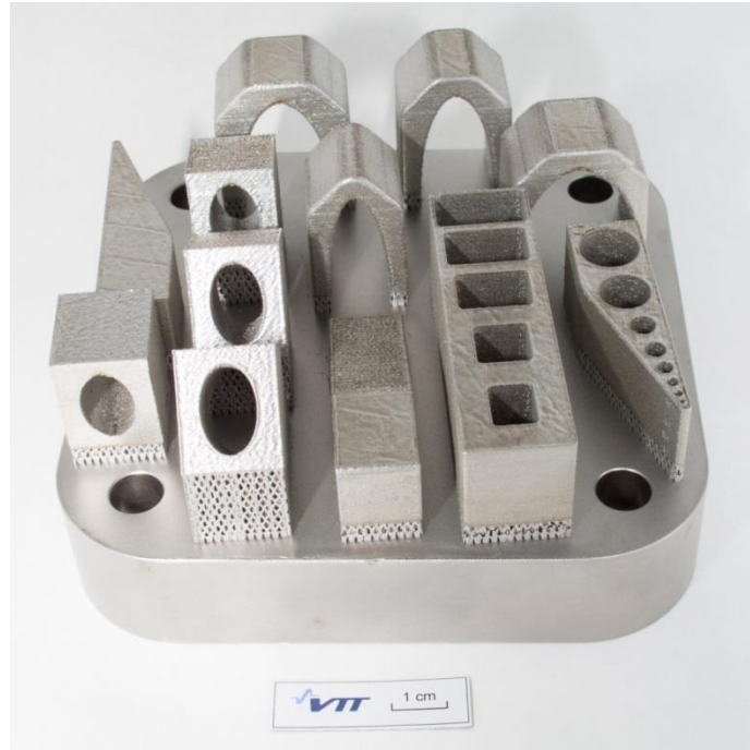
Figure 5. Printed test specimen used in SLM manufacturability tests for creation of design guidelines.
