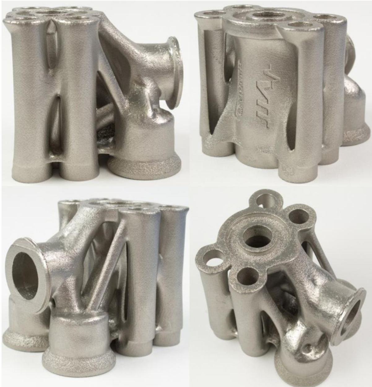
Figure 17. Images of the valve block after support removal and other post-processing procedures.
