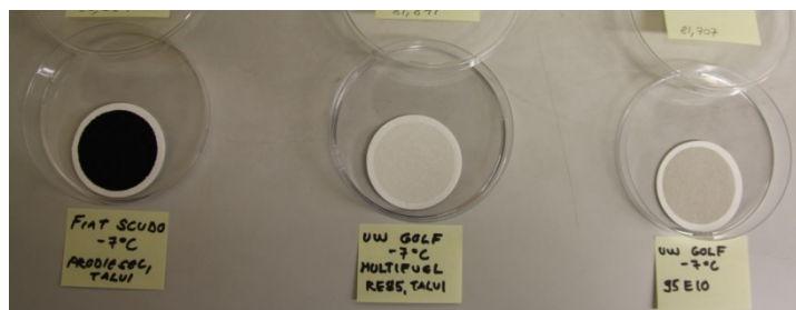
Figure 32. Standard particle collection system and primary Pallflex® TX-40 filter (Ø 47 mm) collected (from left): DI-E2 (Scudo) , E85-E6 , and E10-E6 .
