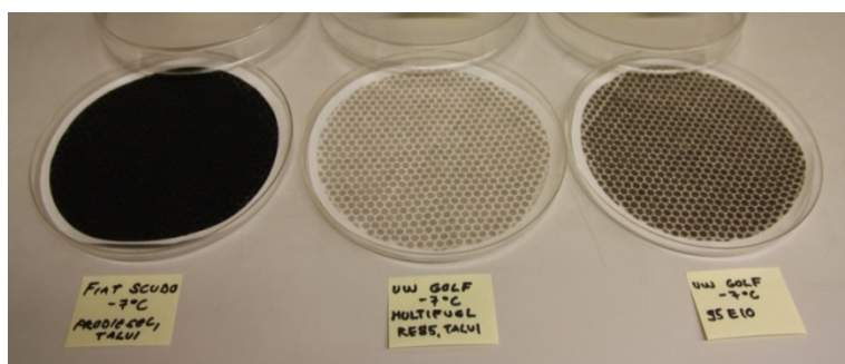
Figure 30. Fluoropore filters after sample collection, from left: DI-E2 (Scudo), E85-E6, and E10-E6.
