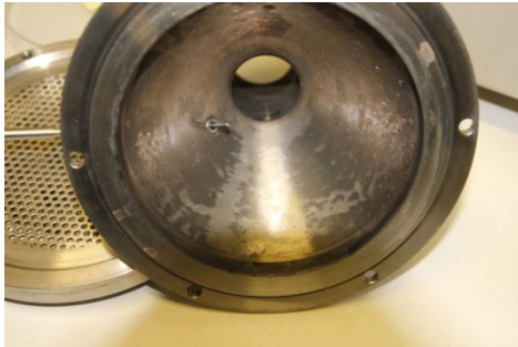
Figure 31. The high-capacity sampler filter holders became wet when collecting samples from E85 .
