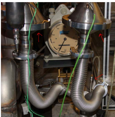
Figure 34. Tenax-tube, Fluoropore filter holders, and gas meter for measurement of sample volumes in Tenax-tubes.
