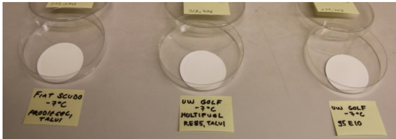
Figure 33. Empore disks after sample collection, from left: DI-E2 (Scudo) , E85-E6 , and E10-E6 .
