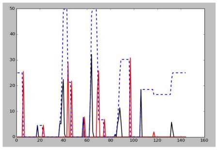
**Figure 6-4.** The optimum heat storage usage. State of charge blue(kWh), recharging heat storage in black(kW) and discharging heat storage in red(kW).
