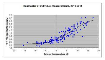
Figure 3-1. Heat pump measurements (Zdeněk, 2011)
