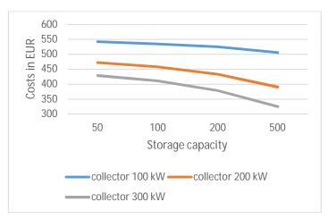
Figure 6-2. Operation cost results with different collector and storage capacity
