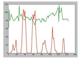
Figure 6-3. Heat load (green) with a 100 kW solar collector simulated output (red)
