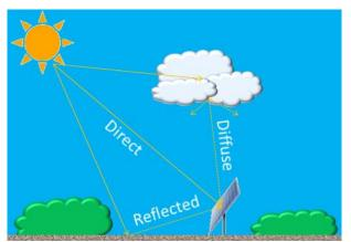
Figure 2-1. Radiation components on tilted panel surface.
