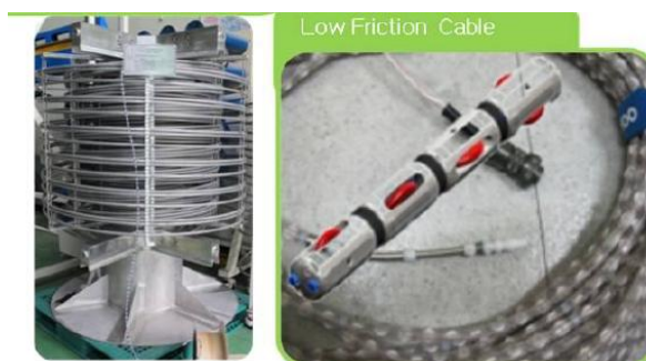
Figure 22. On the left laboratory construction of the SMART Helical SG and on the right its In-service inspection tests with ET bobbin coil [Seo, 2013].
