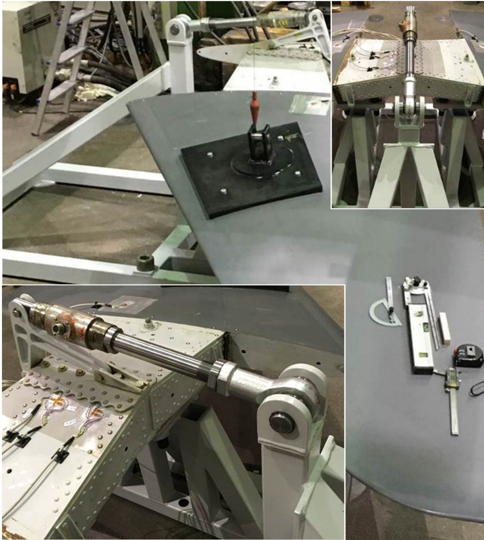
Figure 29: Aligning the upper attachments of the test bench. Figure by courtesy of VTT Ltd.
