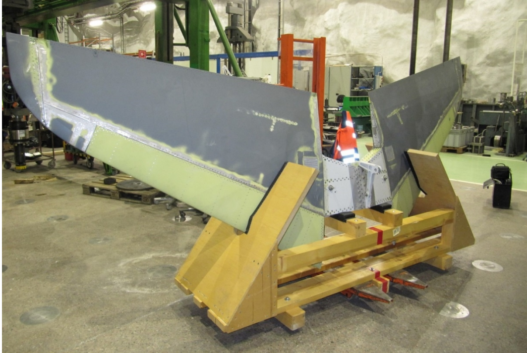
Figure 25: The FINAF Hawk Mk.51/51A/66 Tailplane (LYK45). Figure by courtesy of the FINAF and VTT Ltd.
