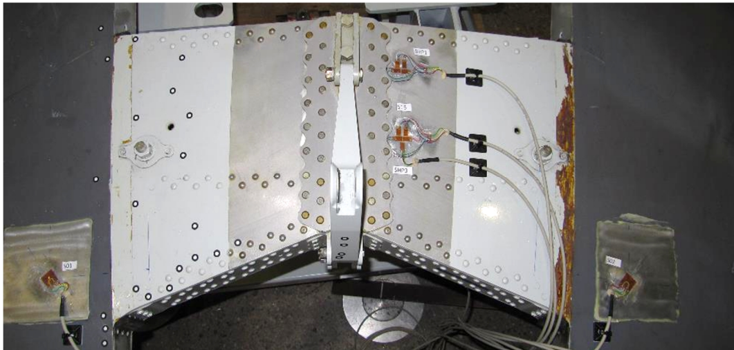
Figure 31: Strain gauges on top of the tailplane. Figure by courtesy of VTT Ltd.
