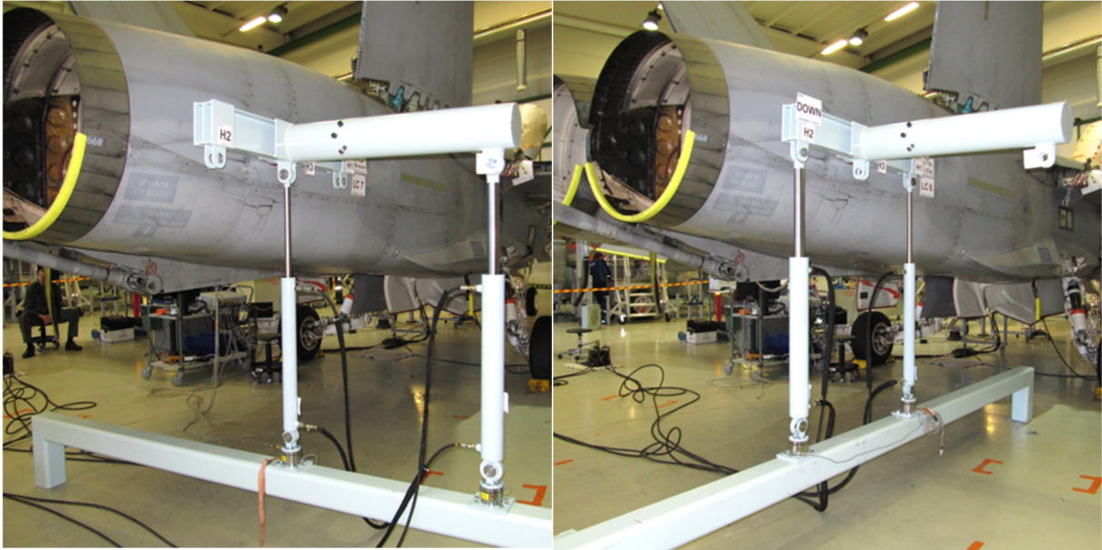
Figure 19: Mechanical calibrations of the HN-416 Bootstrap area. The tool providing bending (left) and torque (right) is manufactured by Patria Aviation. Figure by courtesy of Patria Aviation and VTT Ltd.
