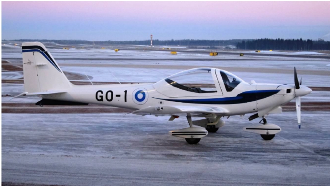
Figure 5: Grob G 115E primary trainer aircraft. Figure by courtesy of the FINAF.
