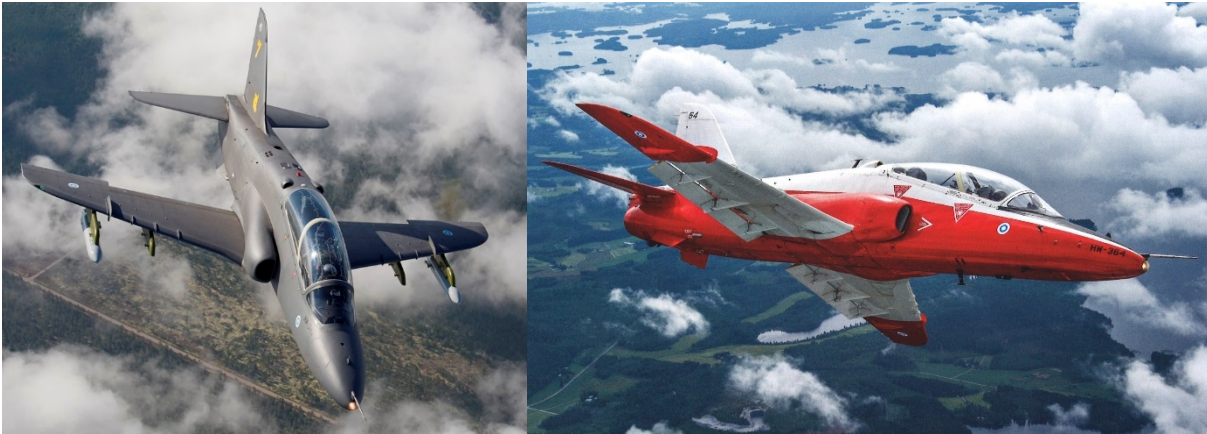
Figure 6: BAE Systems Hawk Mk.51A (left), and Mk.66 (right) advanced jet trainer. Figures by courtesy of the FINAF.
