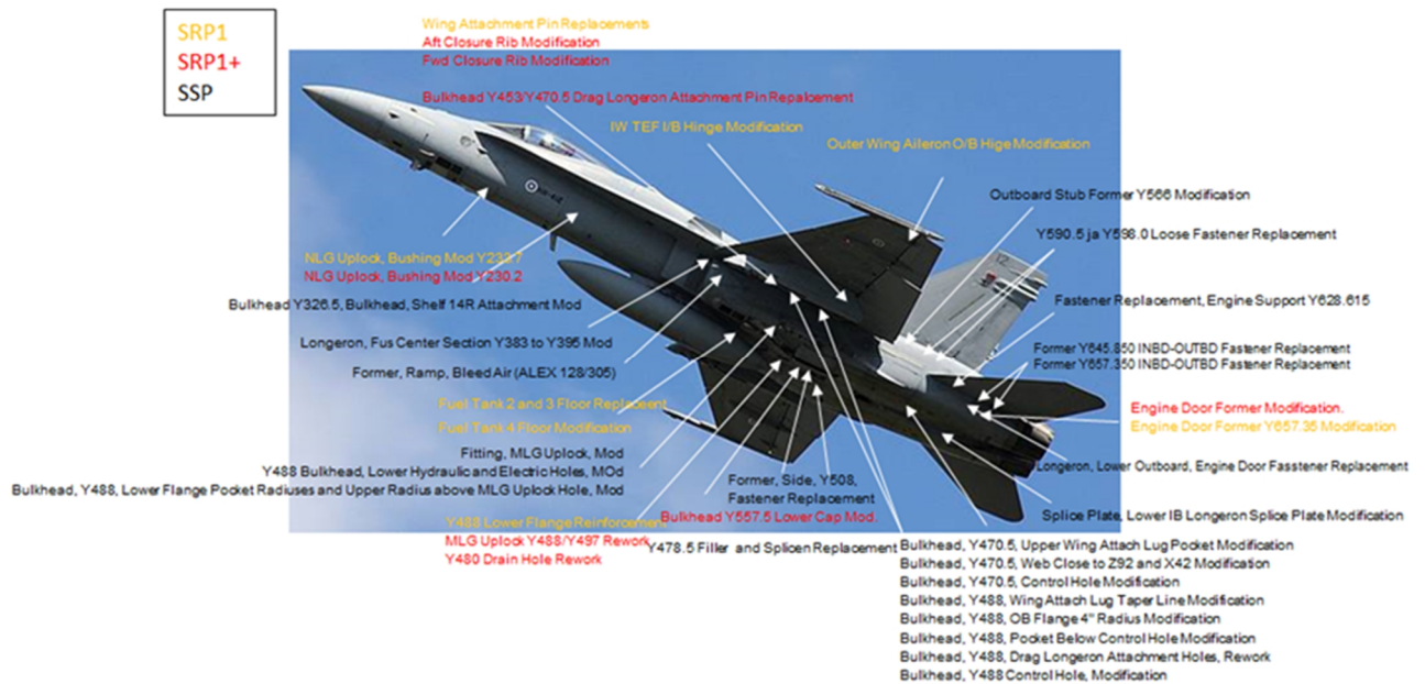
Figure 24: The overview of the SRP1, SRP1+ and SSP modification locations. Figure by courtesy of Patria Aviation.
