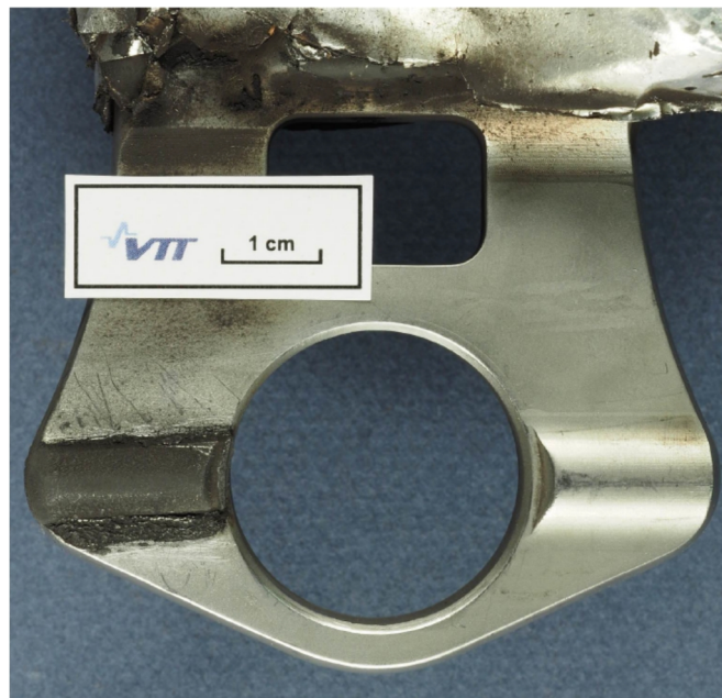
Figure 49: An overview of the thermal sprayed flange prior to machining. Picture courtesy by VTT Ltd.
