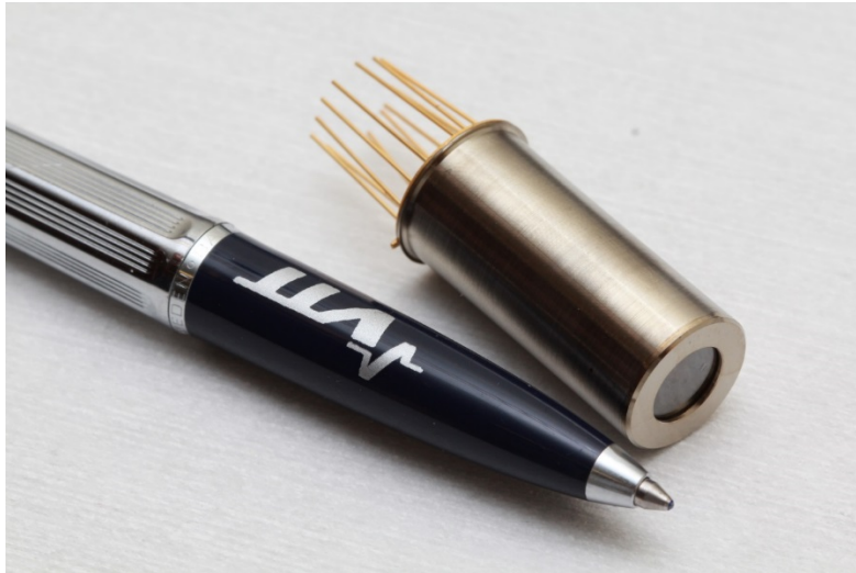
Figure 10. First mock-up module showing the form factor of the packaged MIREGAS light source.
