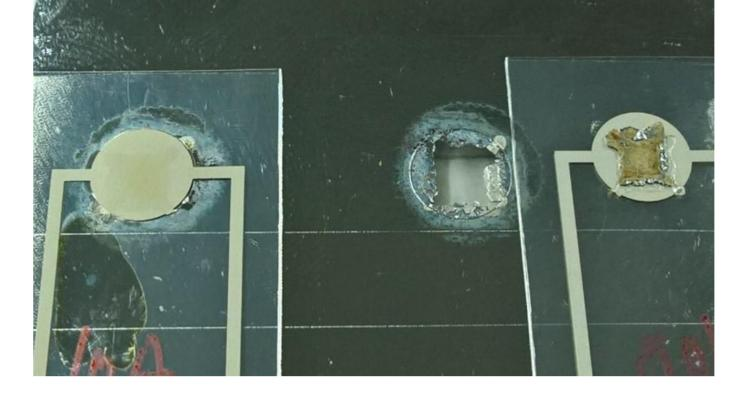
Figure 3. Failure mechanism at the interconnection area in 85°C/85RH% test
