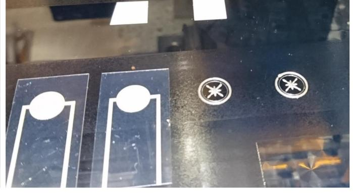
Figure 2. Flexible connectors assembled on OLED foil with conductive adhesive interconnections.
