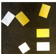
Figure 5.32. Yellow/brownish punches for the 2.5%S fuel after the EC/OC temperature program. Typically punches should be white after the EC/OC analysis.
