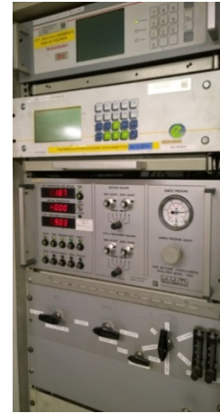
Figure 4.1. Analysers for measuring CO, HC, NO x , CO 2 and O 2 emissions.
