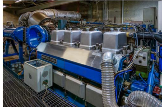
Figure 3.1. VTT's medium-speed engine, Wärtsilä Vasa 4R32 LN.
