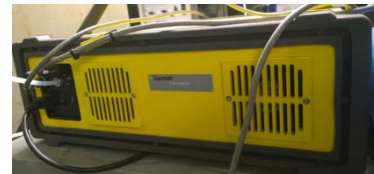
Figure 4.2. The FTIR analyser for on-line multi-component analysis of gaseous emissions.
