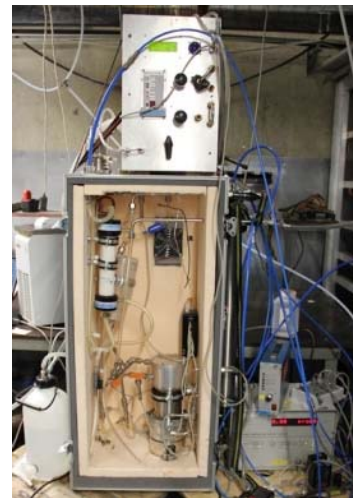
HTDMA: the first DMA on top, the 2nd DMA and CPC below.
